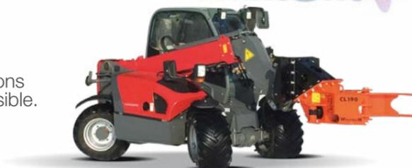
**3** **Cutting mechanism** features replaceable, high-strength knife. Easy to sharpen, rugged and insensitive to dirt.
