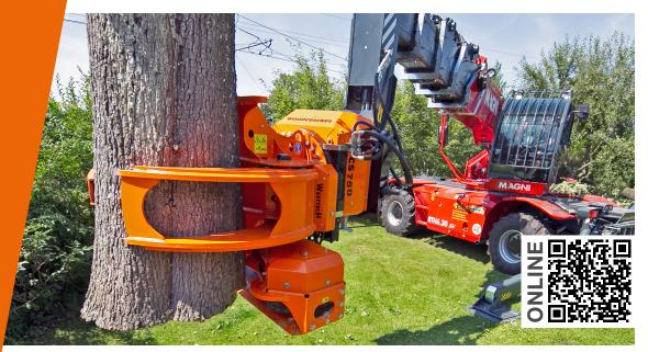
The grip saw for smart attachment to the Roto-Teleloader.
