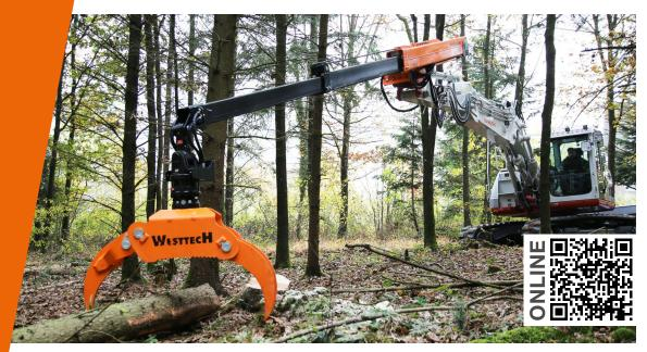
The telescope stage for excavators to increase the reach without any conversion work.
