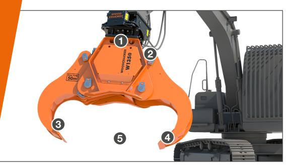
Continuously swivelling rotator with two drive motors as an optional accessory for flexible use. (W1350 & W1800)
