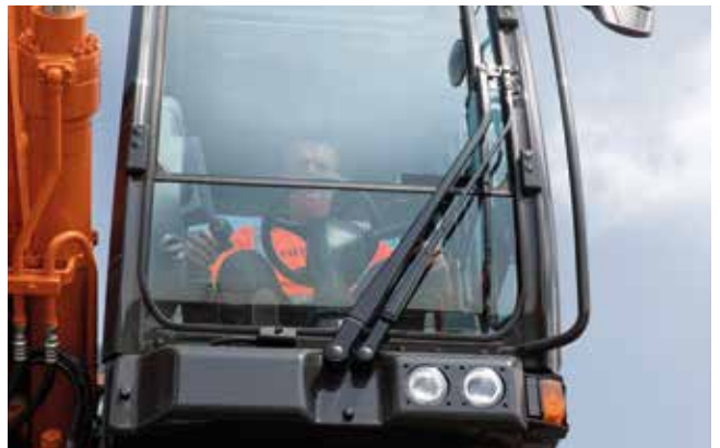
Wider wiper design provides greater visibility.
