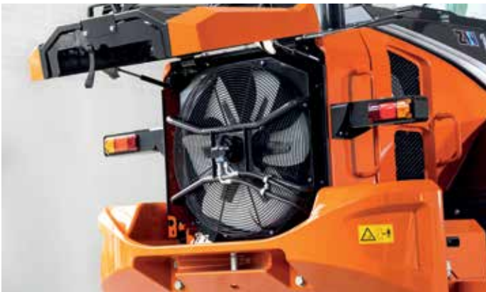
Intelligent fan operation system prevents radiators clogging.
