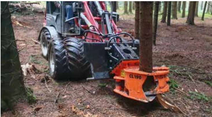
Woodcracker® CL cuts weak wood up to 40 cm.
