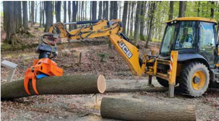
Sturdy and low-wear woodgripper with saw unit.
