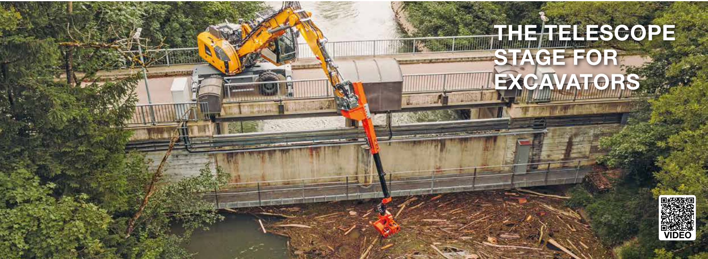
Work range extension up to 6,35 m.
