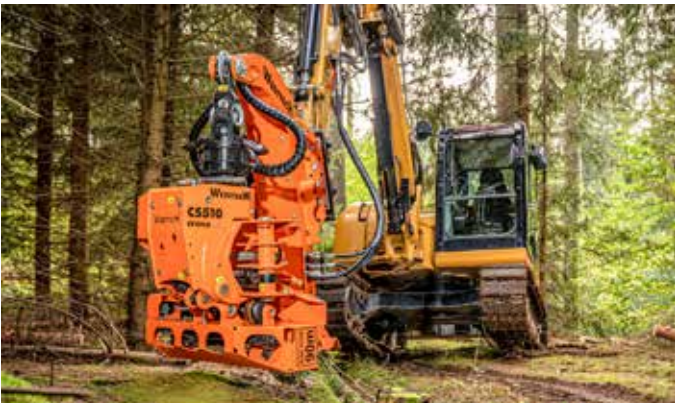
The walking foot allows the excavator to move along, when cardanic machines are attached.
