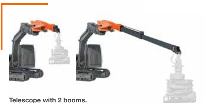
Telescope with 2 booms.
