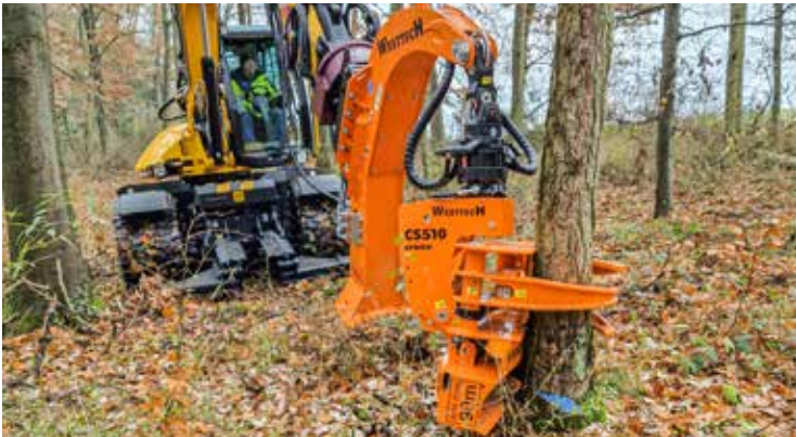
Walking foot with Woodcracker® CS510 crane.
