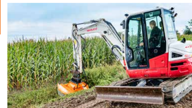
Mulcher at slope maintenance.
