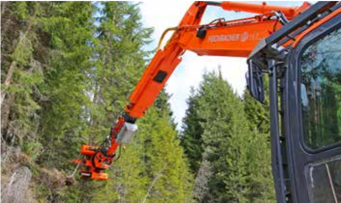
Attachment coupler with Woodcracker® C250.
