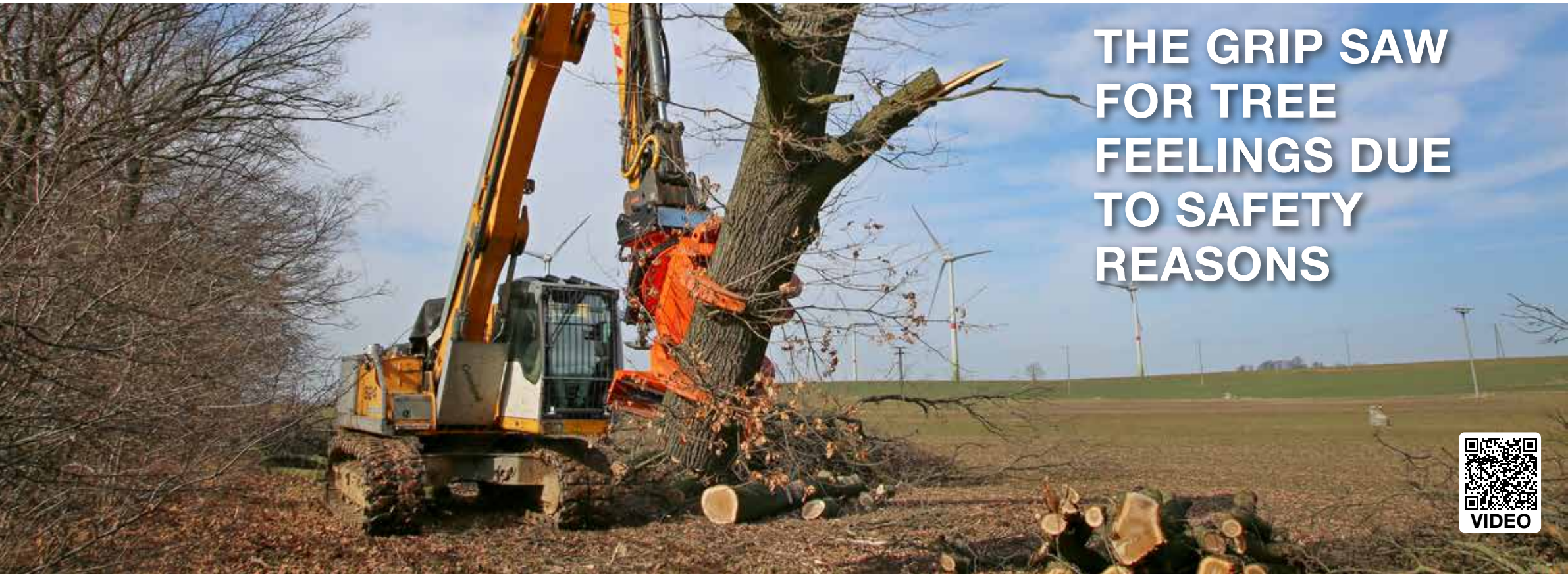
The strong grippers hold the tree firmly.
