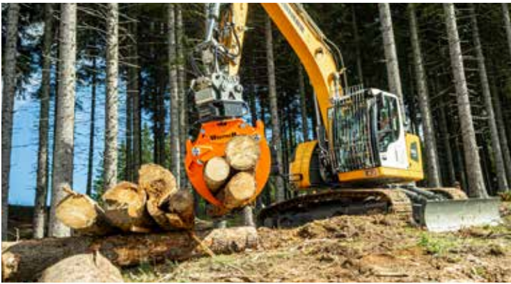
Gripper opening stroke 1270mm.
