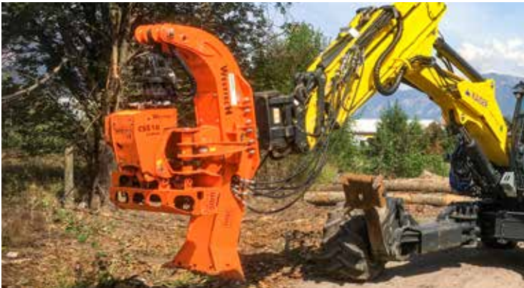
Walking foot on a walking excavator Kaiser S12.
