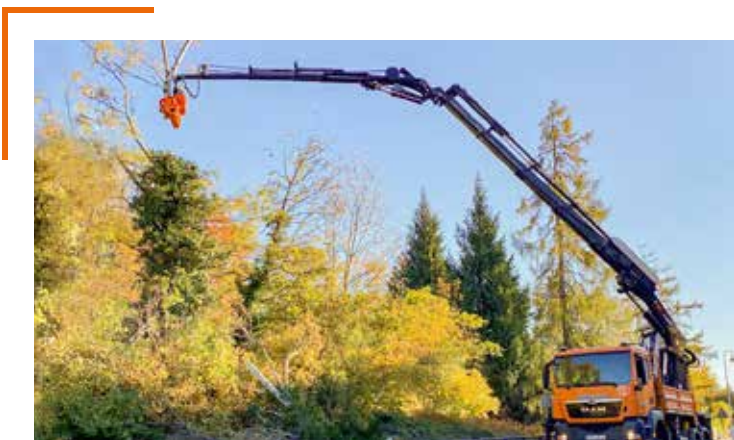
Woodcracker® CS510 crane and Fly-Jib on the Fellertruck.
