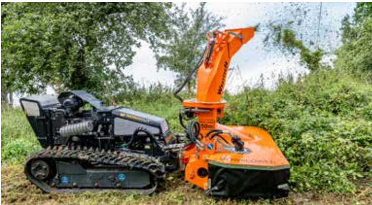
The Mowblower® can be mounted to a remote-controlled mower.
